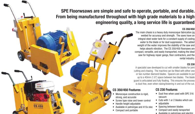
The main chasis is a heavy duty monocoque fabrication jig welded for accuracy and strength. The saws have an integral steel water tank for a constant supply of cooling water to the blade or for dust suppression. The added weight of the water improves the stability of the saw and helps absorb vibration. The CS 350/450 floorsaws are compact, versatile, and easily transported, making the ideal saw for highway repair gangs, floor contractors, and the rental industry.
