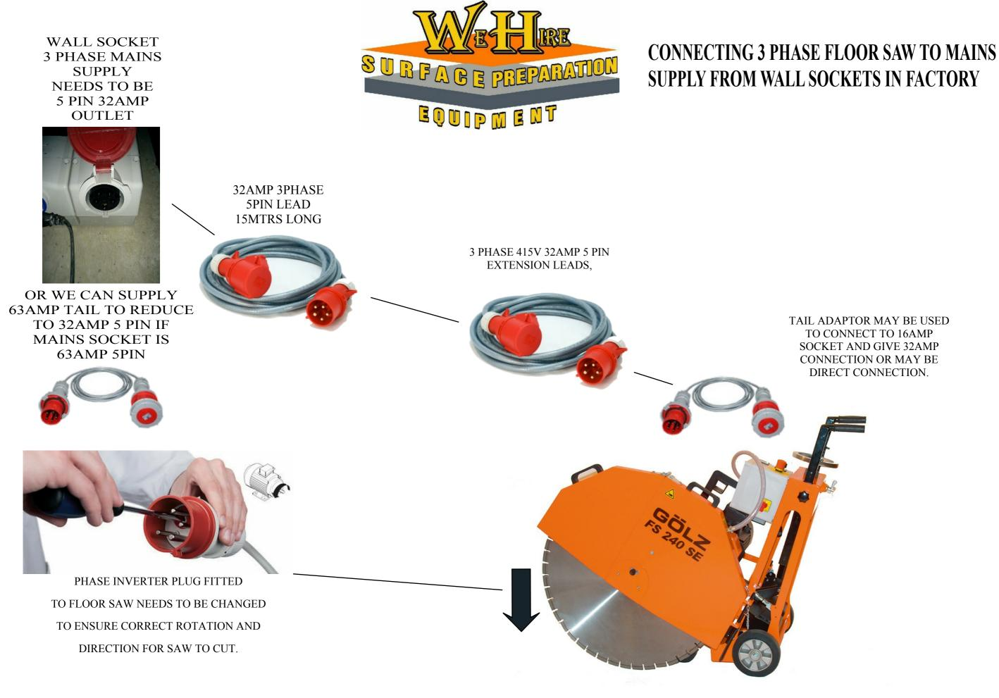
TAIL ADAPTOR MAY BE USED TO CONNECT TO 16AMP SOCKET AND GIVE 32AMP CONNECTION OR MAY BE DIRECT CONNECTION.
