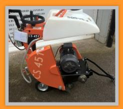
Specification Motor 5.5kW Power 7.5Hp Maximum Blade Capacity 18"/450mm Maximum Cutting Depth 165mm Weight 105kg Requires Min 15kva Generator The CS451-E is highly manoeuvrable and easy to use, enabling it to be used for a wide variety of internal and external cutting applications.
